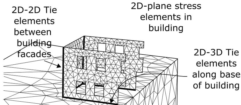
**Figure 3.7:** Complex analysis using Lagrange tie elements.
