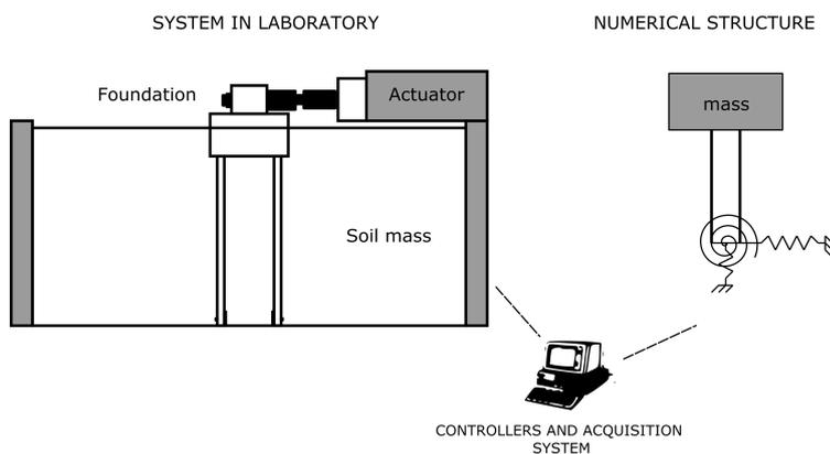
**Figure 2.7:** Configuration for HS of a structure-foundation-soil system.
