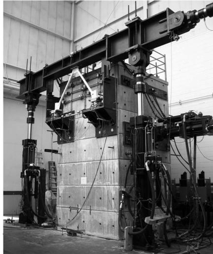
**Figure 3.10:** Actuators configuration for a V-Brace testing.
