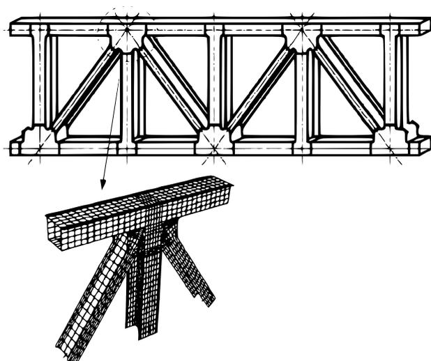
Figure 2.1: Detailed model for local analysis of a truss connection.
