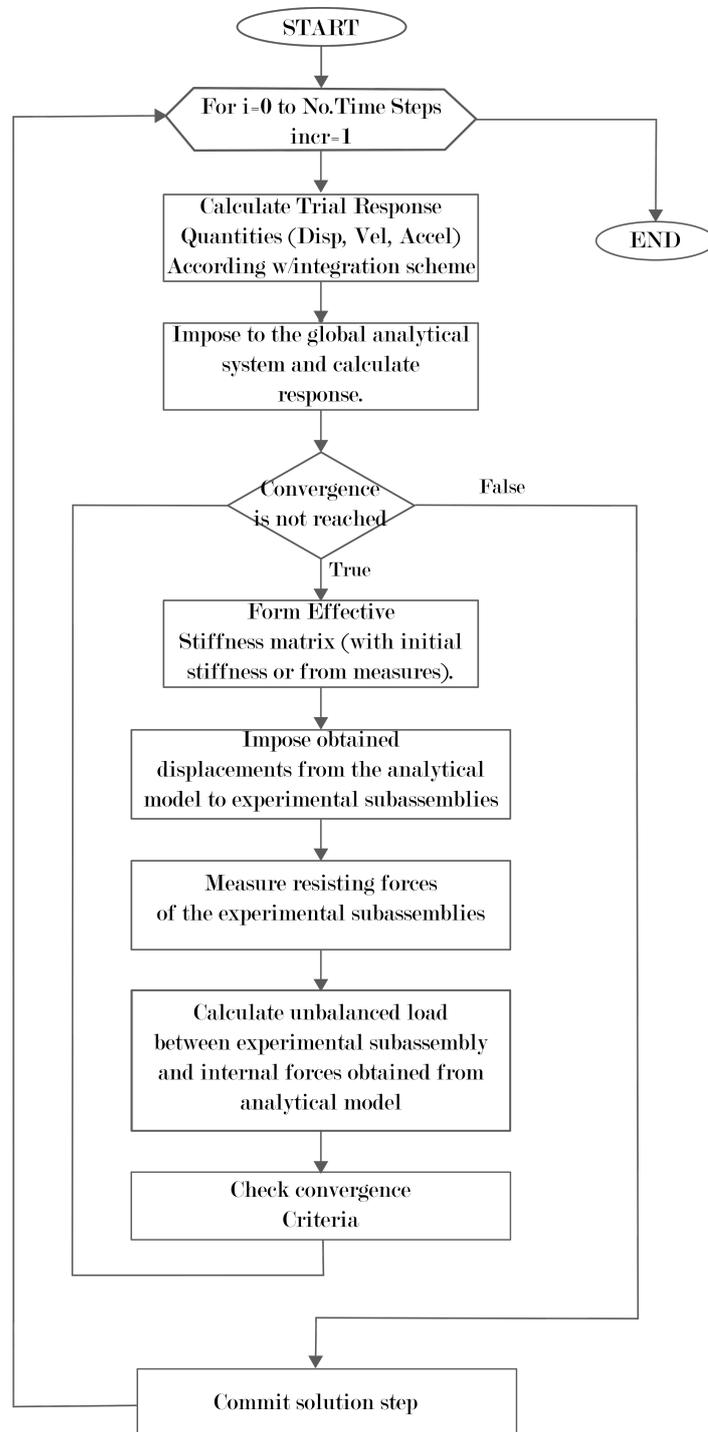
**Figure 3.11:** Classic Hybrid Simulation testing procedure flowchart.
