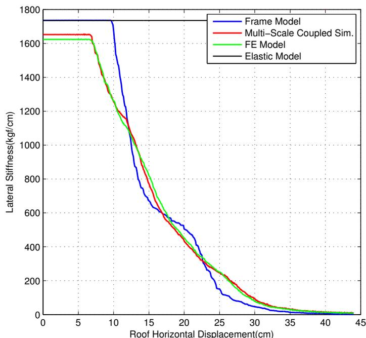
**Figure 5.7:** Decay of the lateral stiffness of the 3 models for the two bay- three story steel frame, during the pushover analysis.
