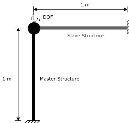
**Figure 4.9:** Beam-Column structural model for numerical coupled analysis.
