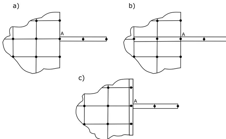
**Figure 3.6:** Connection of a 2D beam with a mesh of 4 node plane-stress elements. a) Hinge mechanism (No moment transferred at point A). b), c) Moment is transferred between the beam and the plane mesh A.
