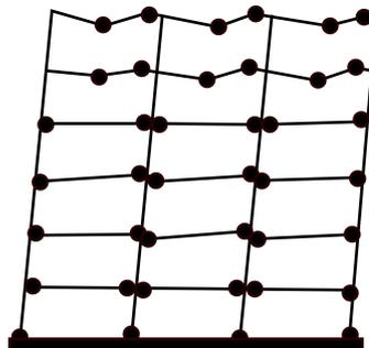
**Figure 1.1:** Plastic hinges model for a plane frame
