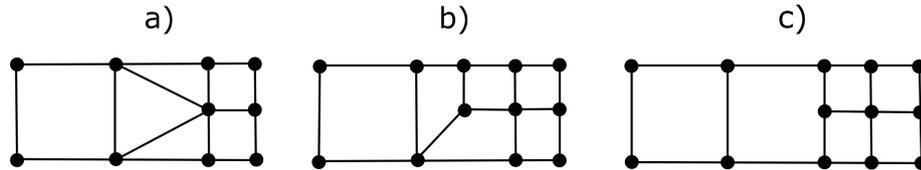
**Figure 3.5:** Mesh transition methods for plane problems.
