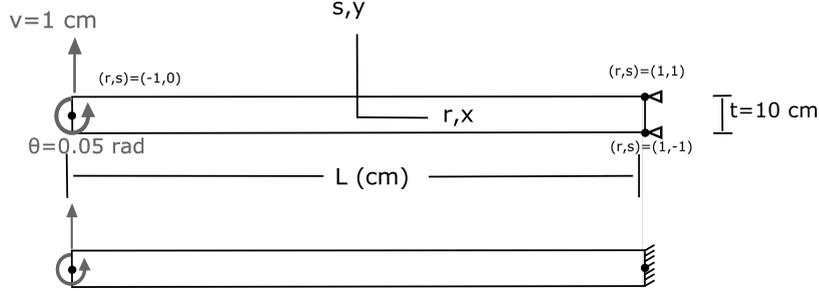
**Figure 4.3:** Displacement imposition configuration for the bending test and internal forces diagrams for its analogue frame (bending moment and constant shear).
