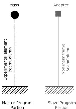
**Figure 4.11:** Cantilever structural model for numerical coupled analysis.
