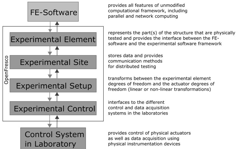
**Figure 3.12:** OpenFresco framework components to conduct an HS.
