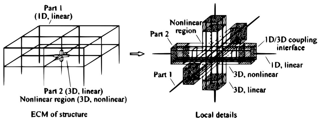
Figure 2.2: Modeling of a three-dimensional frame with the Element Coupling Method.
