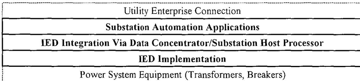
Figure 4 – Levels of Substation Integration and Automation
