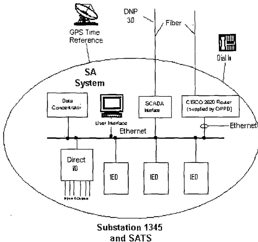
Figure 6 – Substation 1345 and SATS Integration Architecture
