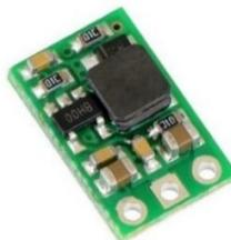
Fig. 2.16 Pololu 9V Step-Up Voltage Regulator U3V12F9
