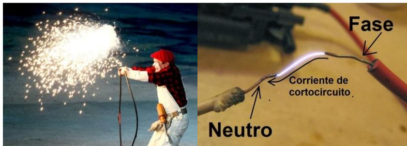
Imagen 56. Cortocircuito. Obtenido de: izq. <http://img.terra.com.br/i/2010/02/28/1460786-7882-atm14.jpg> el 06/08/2015, der. [http://1.bp.blogspot.com/AmnD736p\\_f4/Uucjr\\_hJHMI/AAAAAAAAxQ/pnnsT3HVkF0/s1600/cortocircuito.jpg](http://1.bp.blogspot.com/AmnD736p_f4/Uucjr_hJHMI/AAAAAAAAxQ/pnnsT3HVkF0/s1600/cortocircuito.jpg) el 06/08/2015
