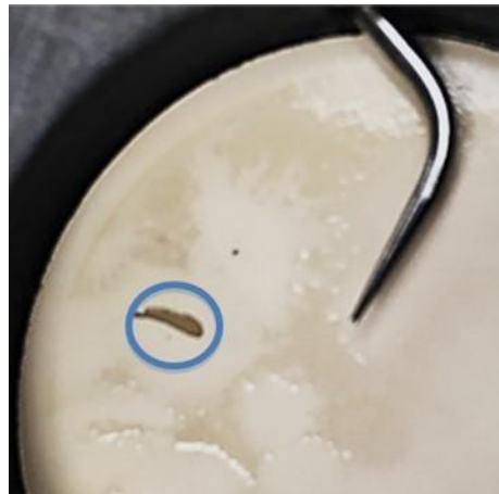
Figure 4. Damaged surface of a 0.8 µm ceramic membrane produced by a UDS tip 10P exceeding the exposure time (longer than 30 minutes).
