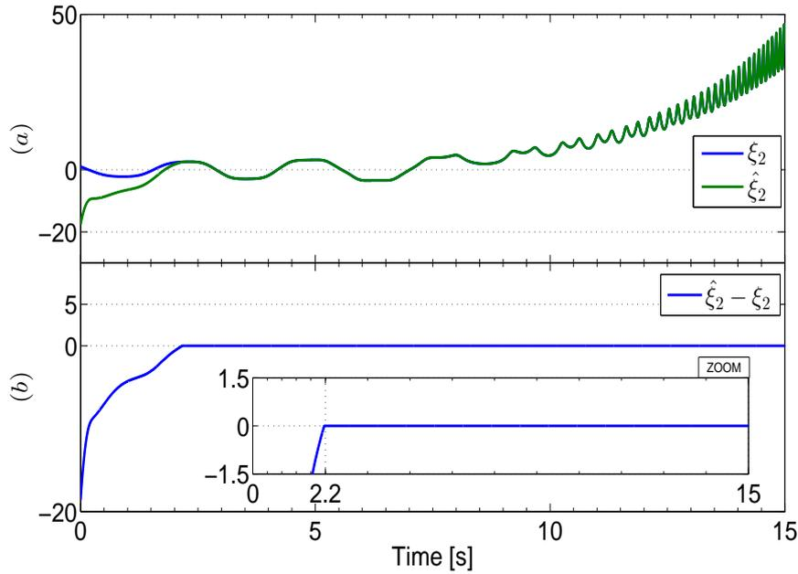
FIGURE 3.4: (a) The real states  $\xi_2$  on (3.2) and their estimation state  $\hat{\xi}_2$ . (b) The estimation error  $\hat{\xi}_2 - \xi_2$
