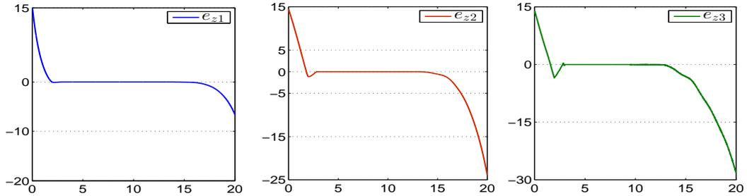
FIGURE 2.6: The estimation errors  $e_{z1} = z_1 - x_1$ ,  $e_{z2} = z_2 - x_2$ ,  $e_{z3} = z_3 - x_3$  of the sliding-mode differentiator (2.24)
