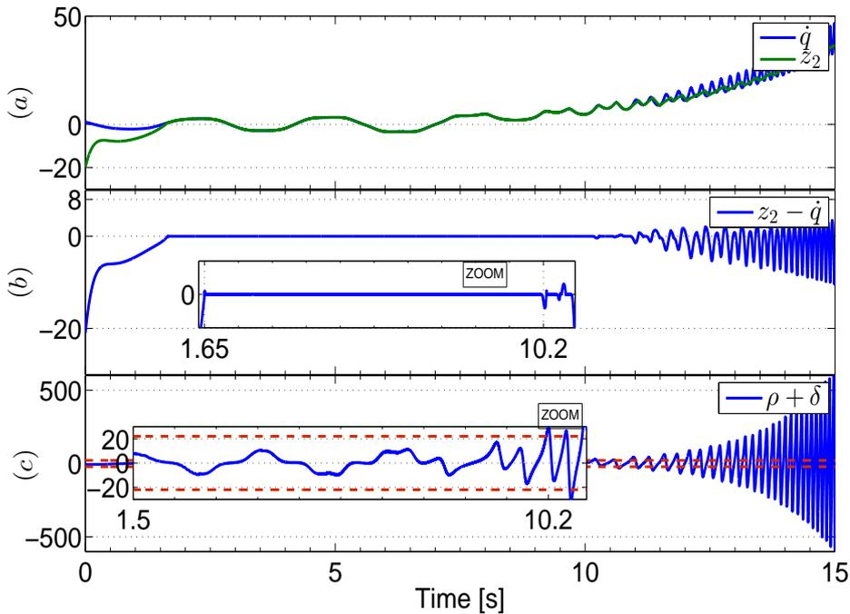
FIGURE 3.1: (a) The estimation state  $z_2$  of differentiator (3.3) and the real state  $\dot{q}$  of (3.2). (b) The estimation error  $z_2 - \dot{q}$ . (c) Nonlinearity and the perturbation  $\rho + \tilde{\delta}$  overcome the gain 20
