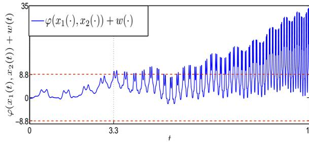
FIGURE 1.2: The function  $\varphi(x_1(t), x_2(t)) + w(t)$  exceeds the gain 8.8 of the discontinuous term in the differentiator (1.3)
