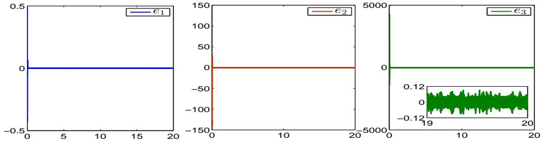
FIGURE 2.8: The estimation errors  $e_1 = \hat{x}_1 - x_1$ ,  $e_2 = \hat{x}_2 - x_2$ ,  $e_3 = \hat{x}_3 - x_3$  of the proposed observer (2.17)
