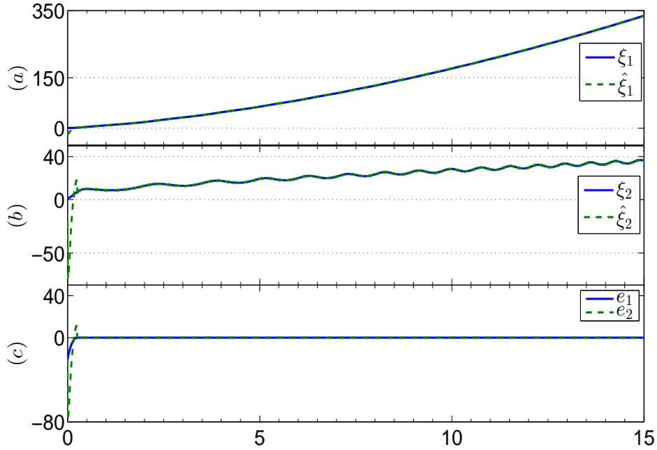
FIGURE 3.5: (a)-(b) The real states  $\xi_1$ ,  $\xi_2$  and their estimation states  $\hat{\xi}_1$ ,  $\hat{\xi}_2$ , respectively. (c) The estimation errors  $e_1 = \hat{\xi}_1 - \xi_1$ ,  $e_2 = \hat{\xi}_2 - \xi_2$
