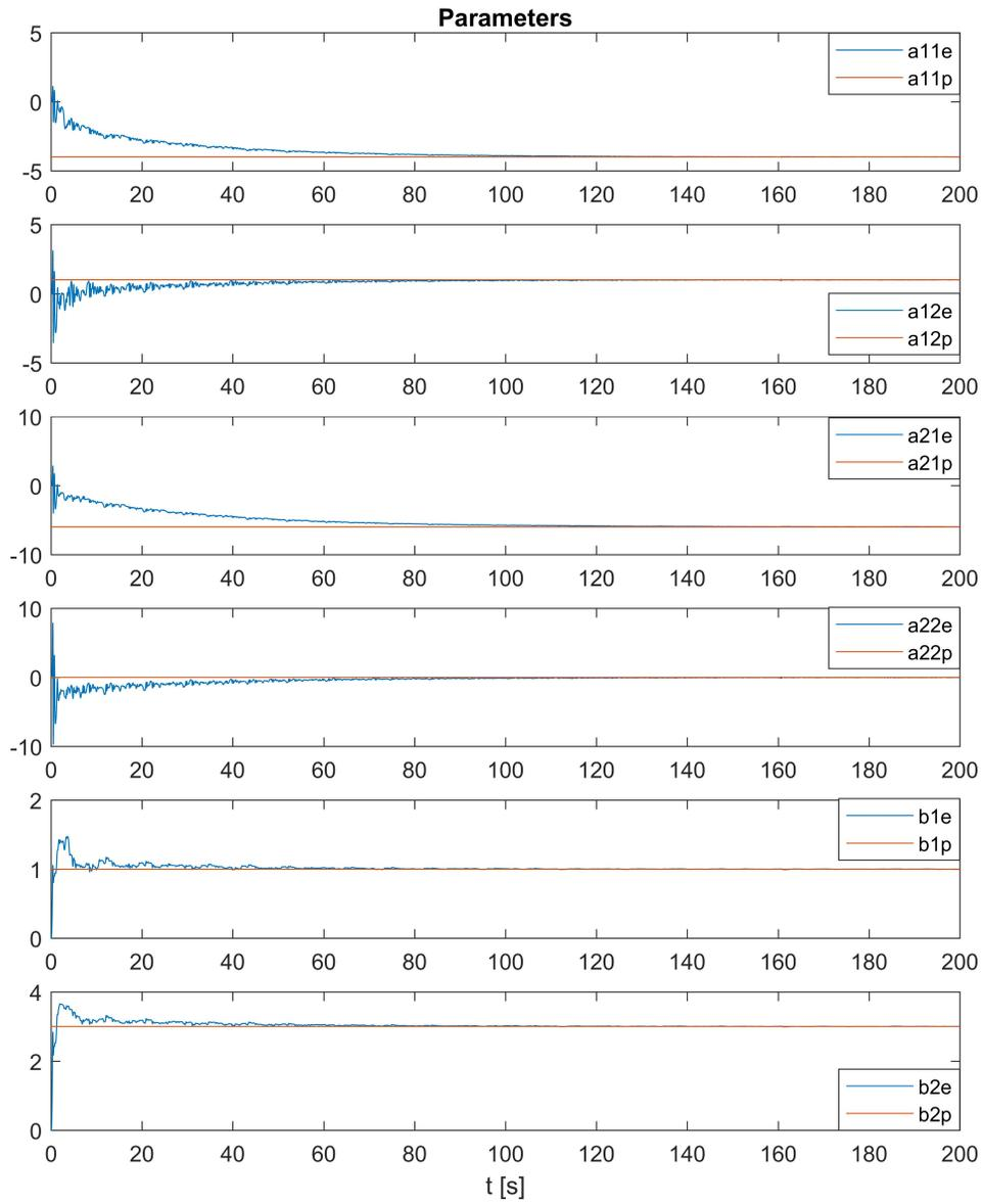
Figure 4.6: Identification scheme with state measurement, parameters estimates, where  $p$  and  $e$  indicates plant and estimate, respectively.
