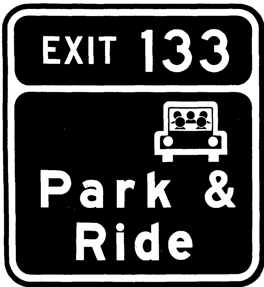
Figure 2-26. Guide sign to park & ride facility. (Freeway).
