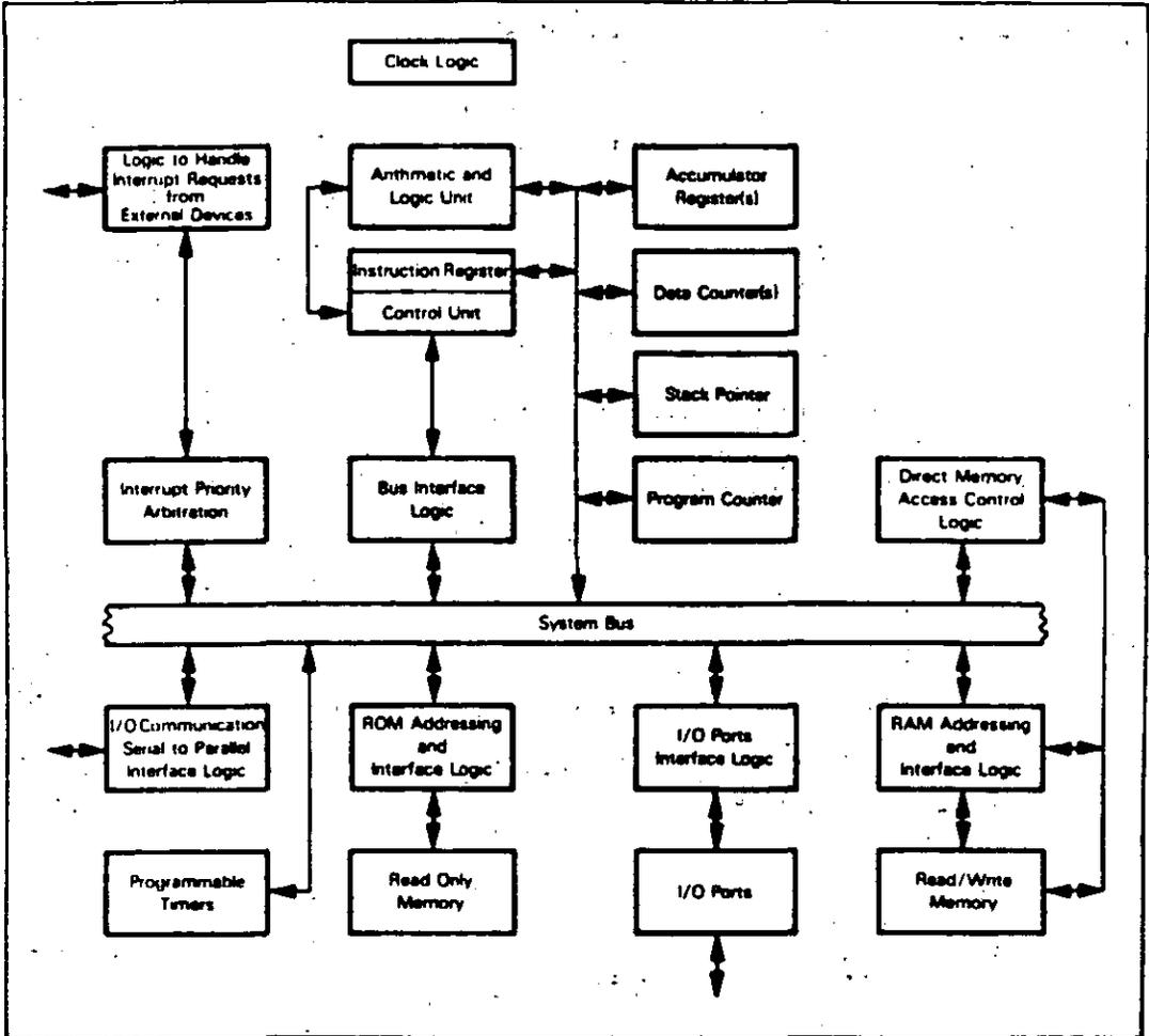
Figure 20-1. Logic of the Intel 8086 CPU
