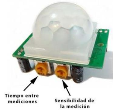
Figura 4. Trimpots del sensor PIR [4].
