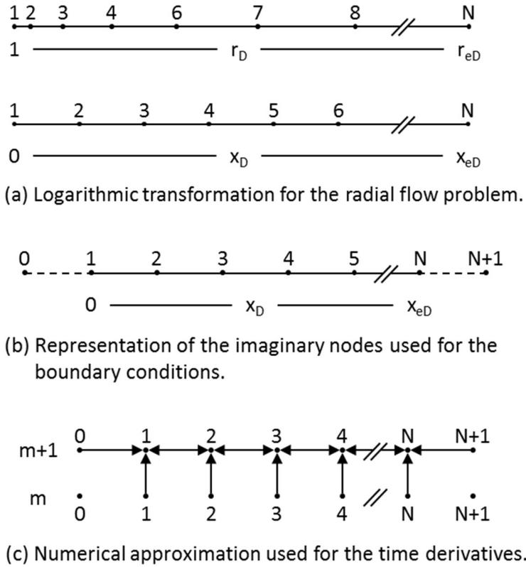
**Figure C. 1. Schematization of the numerical discretization used for radial flow.**
