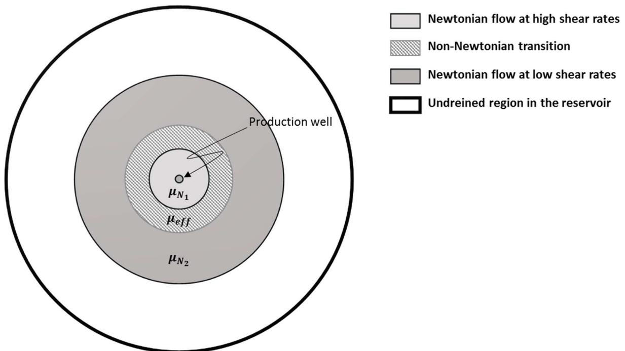
**Figure 4.1. Flow regions in a radial reservoir for a power-law type fluid.**
