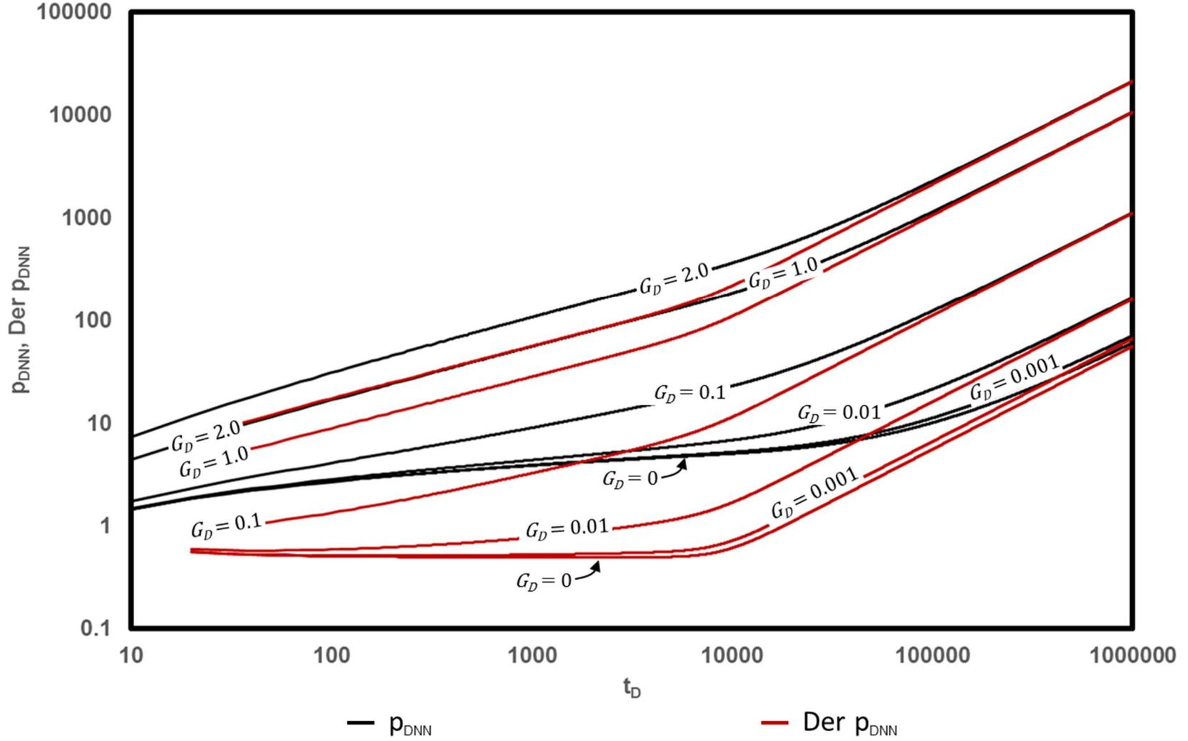
Figure 6.9. Comparison between the values of the dimensionless pressure drop for a Newtonian and a Non-Newtonian Bingham plastic fluid in a finite radial reservoir of  $r_{eD} = 200$  (cases for  $G_D = 0.001, 0.01, 0.1, 1$  and  $2$ ).
