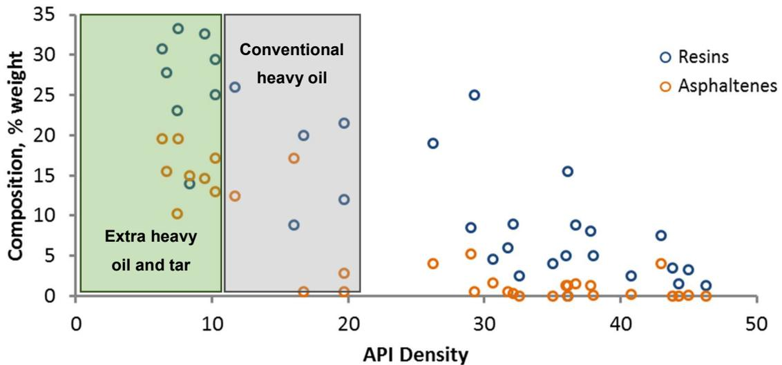
**Figure 1. 2. Correlation between the API density and content of resins and asphaltenes for different oil mixtures<sup>3, 4, 5</sup>.**
