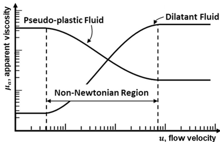
**Figure 2. 1. Apparent viscosity for a power-law type fluid as a function of the flow velocity (after Poon and Kisman<sup>13</sup> and Bondor<sup>31</sup>).**
