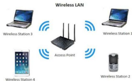
Figura 82 Diagrama de conexiones de una red WLAN [<https://letsmesaytech.blogspot.com/2018/12/wlan-what-is-wlan.html>]
