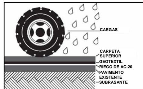
FIG. 2.14 BARRERA PROTECTORA IMPERMEABLE PARA LA SUBRASANTE
