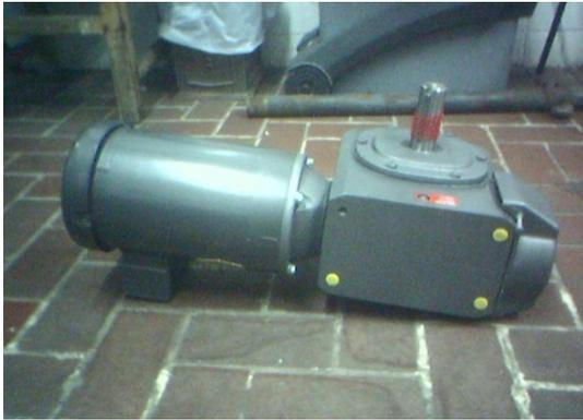
Fig. 5.48. Motorreductor principal
