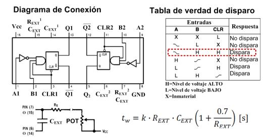
▲ Figura 4.7. Circuito multivibrador monoestable 74LS123.
