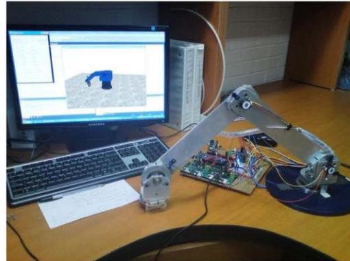
Figure 13. Teleoperation System for experimentation
