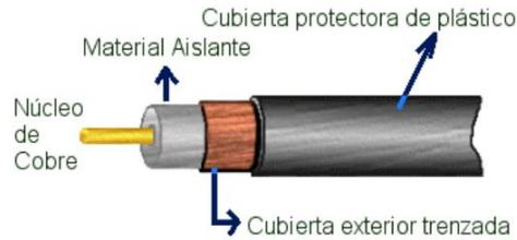
Figura 12 Cable coaxial RG6.
