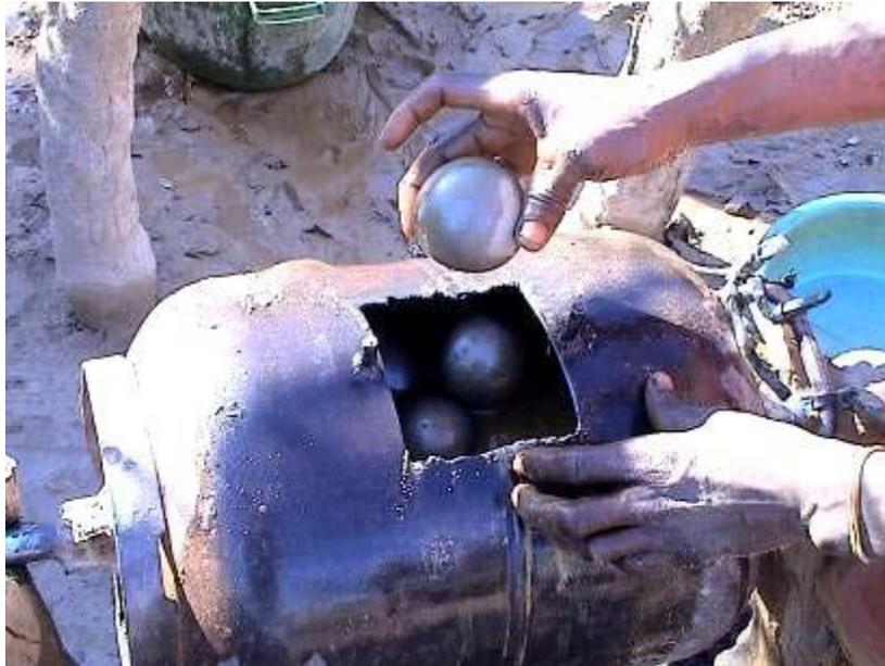
Figura 15 Cargado de bolas (Global Mercury Project, 2006)
