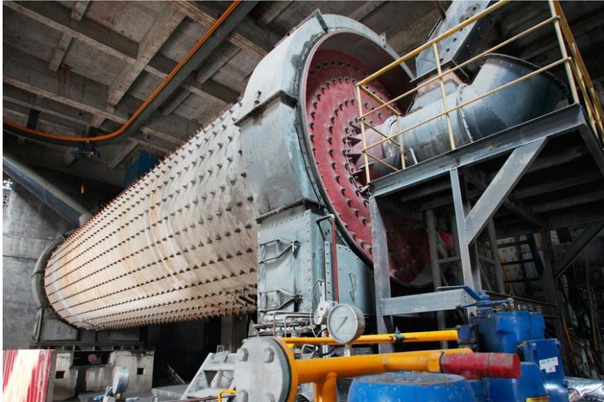
*Figura 179. Molino de bolas (GCP Applied Technologies, 2020).*
