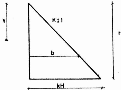
Fig. III.4 Muro triangular.
