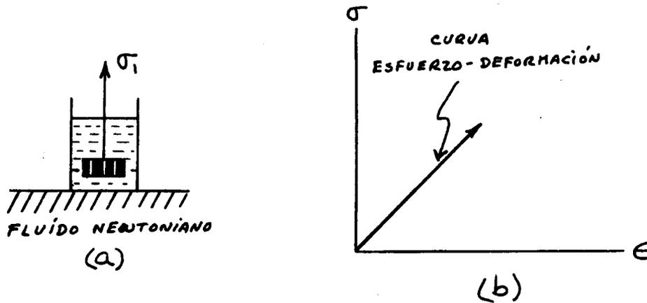
Figura 66.. (a) MODELO REOLOGICO PARA UN MATERIAL VISCOZO.
