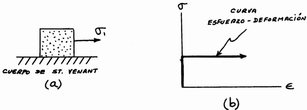
Figura 65. (a) MODELO REOLOGICO PARA UN MATERIAL PLASTICO.
