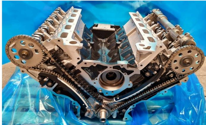
Figura 2. Motor Ford 6.8 V10. [1]
