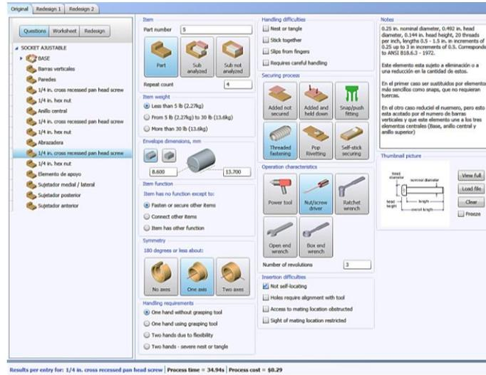
Figura 5.19 Interface del software de DFA [55]
