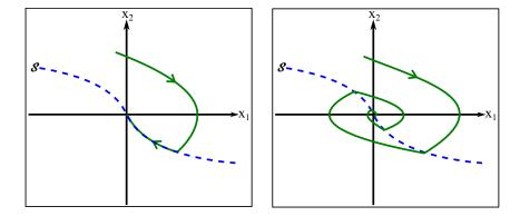
Figure 4.2: Trajectories of (4.2), (4.6). Left: Terminal behavior. Right: Twisting behavior
