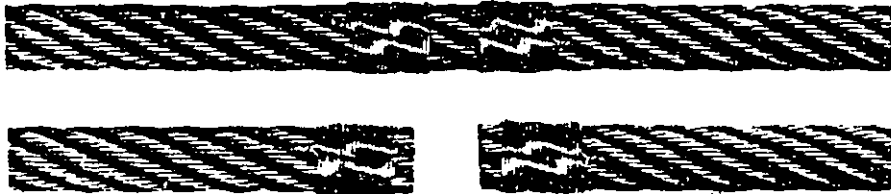
Seizings for Form-Set Steel Wire Ropes before and after cutting.
