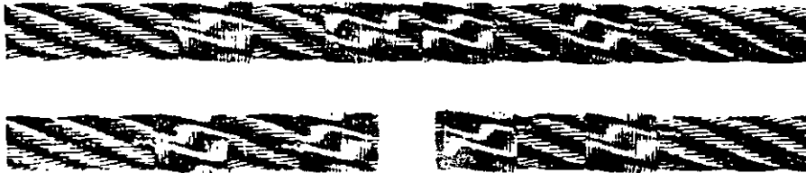
Seizings for non-preformed Steel Wire Ropes \frac{7}{8} in. in diameter and smaller before and after cutting.
