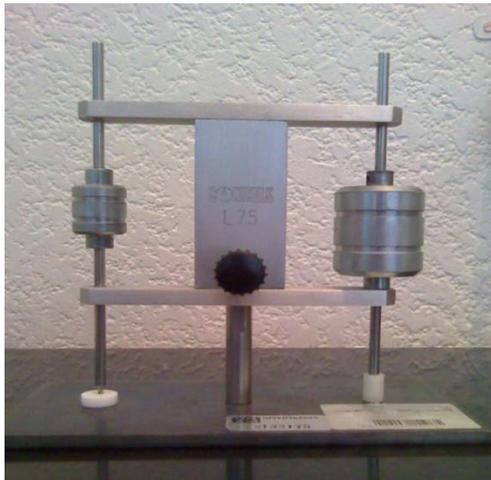
Figura 25. Agujas de Gillmore (norma ASTM C266-89)
