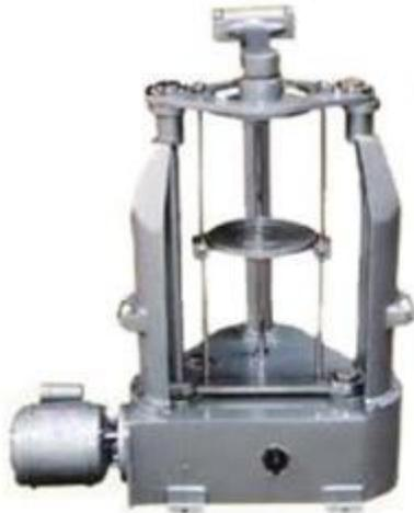
Fig 1.3 Shaker mecánico (“Laboratory mechanical shaker”, Vidiac)
