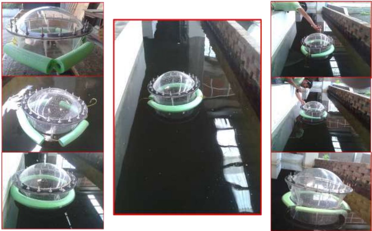
Figure 12. Control test: Bouyancy.
