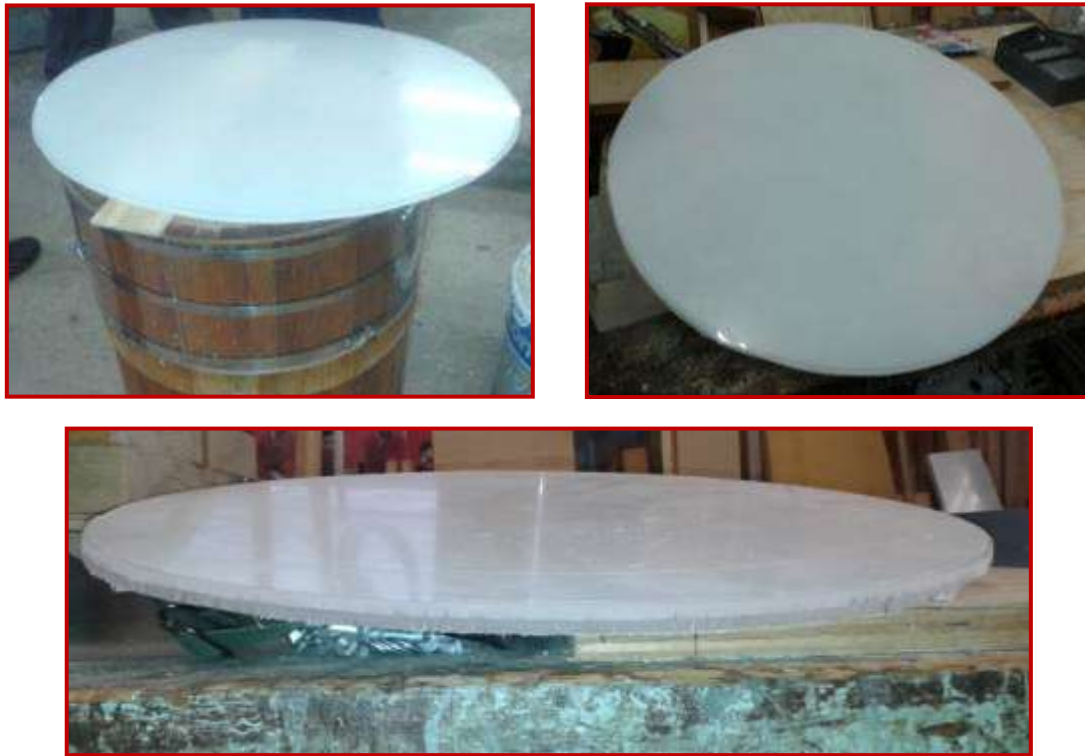
Figure 8. Making of washers for the dome and base of the Static Flux Chamber.
