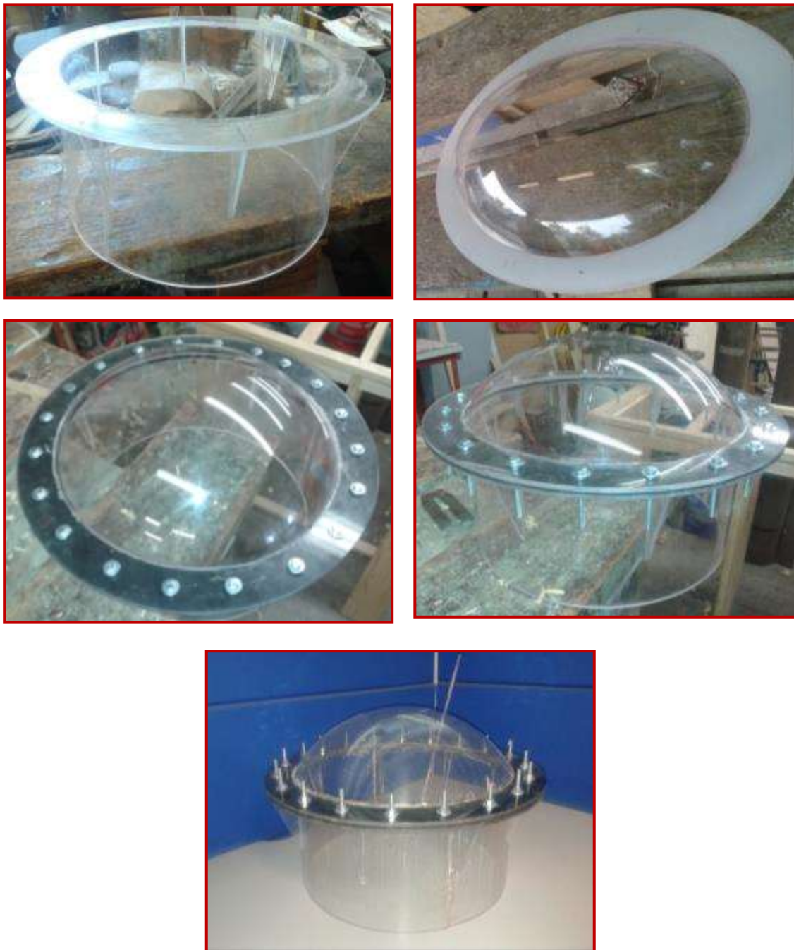
Figure 10. Assembly of Static Flux Chamber.
