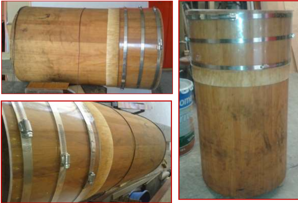
Figure 7. Wooden mold for the acrylic circular base of Static Flux Chamber.
