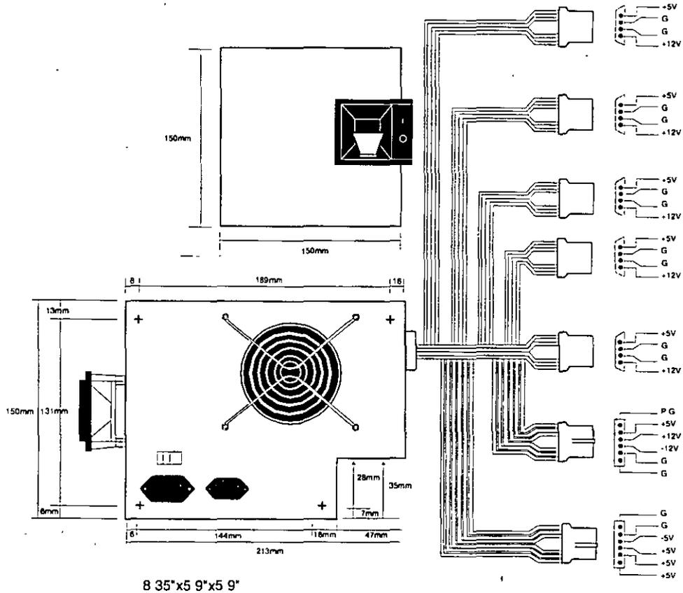
**Figure 8.2.** AT/Desktop form factor power supply.
