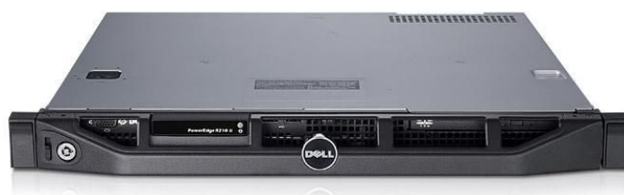
Figura 3.32: Servidor Dell PowerEdge R210
