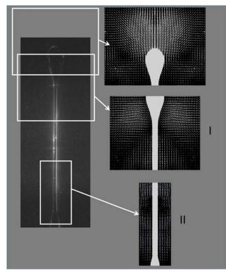
Fig. 10 The deformation of a viscoelastic sol. A (8 ml droplet) is divided into two regions: I (head) and II (tail). PIV measurements are shown for each section
