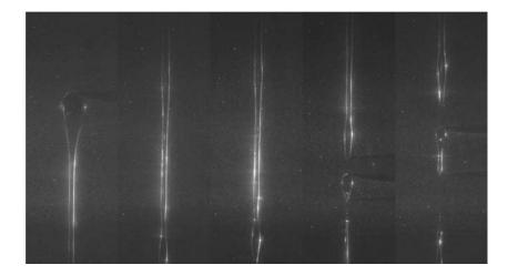
The tail may vary in diameter as it is elongated as the droplet rises. This section may be useful as a possible measure of elongational unidirectional flow or to determine the extensional viscosity of the fluid in the droplet (see for example Cruz-Mena et al. 2002, Rios et al. 2002).
