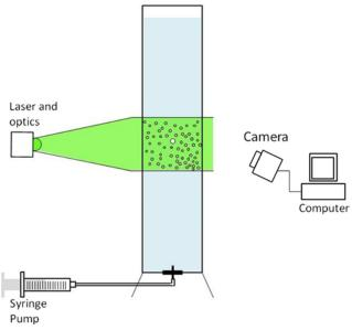
Fig. 1 Experimental setup
