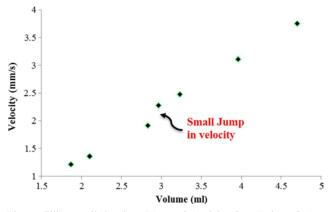
Fig. 6 Silicone oil droplets (Newtonian) rising in a Polyox 0.5 % aqueous solution D (viscoelastic) fluid
