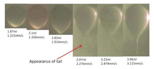
Figure 12 shows the typical behavior of a droplet (solution A) in the Polyox (solution D). The distinct regions are depicted in the photograph.
