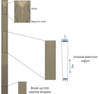
Fig. 12 Schematic description of the observed uniaxial tension on the droplet in the distinct regions of interest
