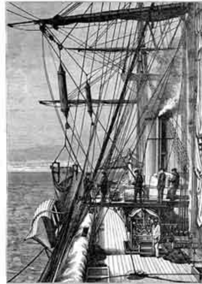
Fig. 12.—Trawling and sounding arrangements on board the Challenger. Figura I.2) *H.M.S. Challenger, muestreando. (Bailey-Herbert, 1953, Viaje del challenger.)
