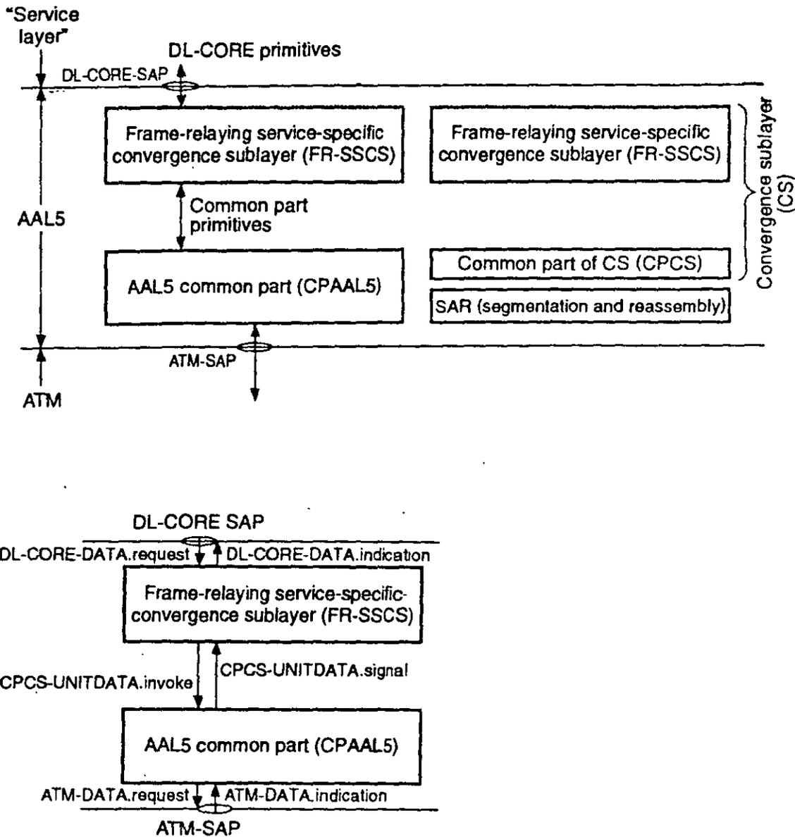
Figure 3.19 AAL5 for interworking of frame relay and ATM (in CPE).
