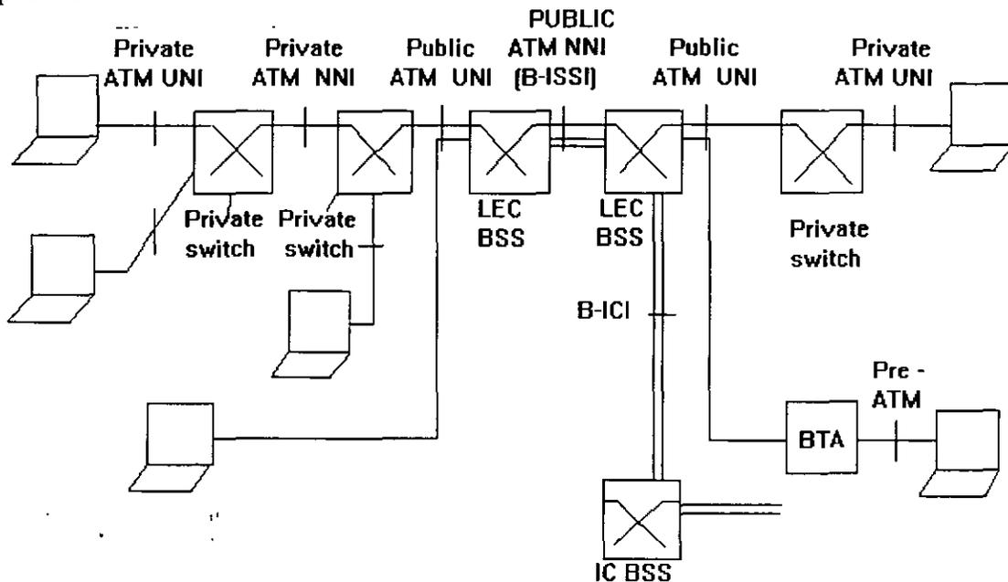
**Figure 1.1** A physical view of an ATM/CRS private/public network. BSS = broadband switching system (B-ISDN switch); BTA = broadband terminal adapter; B-ISSI = broadband interswitching system interface; BICI = broadband intercarrier interface; LEC = local exchange carrier; IC = interexchange carrier.
