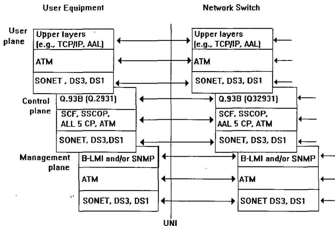
**Figure 1.3** Planes constituting the ATM protocol model.
