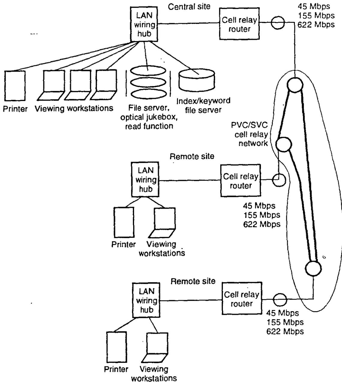
Figure 1.17 Use of ATM/cell relay to support imaging.
