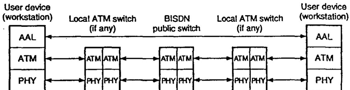
Figure 3.2 The positioning of AAL in CPE.
