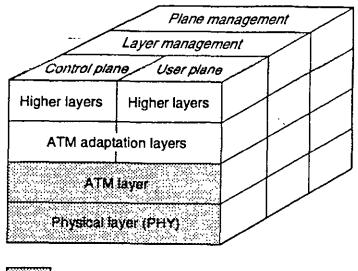
Protocol layers relevant to cell relay service
