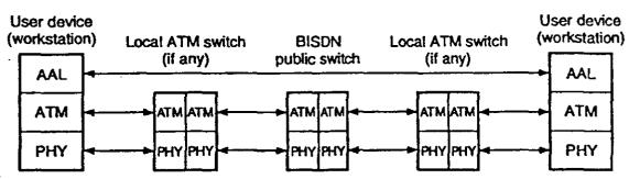
Figure 3.2 The positioning of AAL in CPE.
