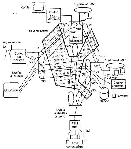
Figure 1.6 Example of use of VPs and VCs in an enterprise network (broadband switches not shown for simplicity). *Note*: VPs and VCs can be preprovisioned (PVCs) or ondemand (SVC whit signaling)
