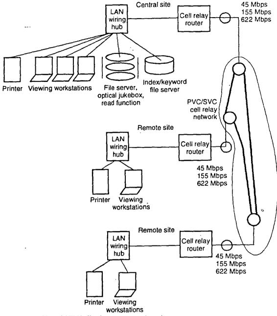
Figure 1.17 Use of ATM/cell relay to support imaging.
