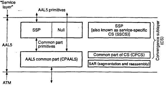
Figure 3.14 Structure of AAL Type 5.
