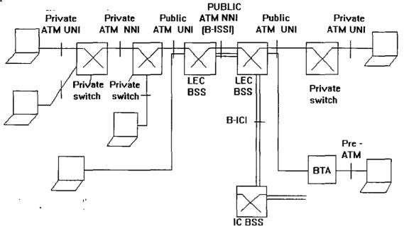
**Figure 1.1** A physical view of an ATM/CRS private/public network. BSS = broadband switching system (B-ISDN switch); BTA = broadband terminal adapter; B-ISSI = broadband interswitching system interface; BICI = broadband intercarrier interface; LEC = local exchange carrier; IC = interexchange carrier.
