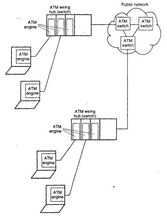
Figure 1.14 Example of usage of ATM in an enterprise network.
