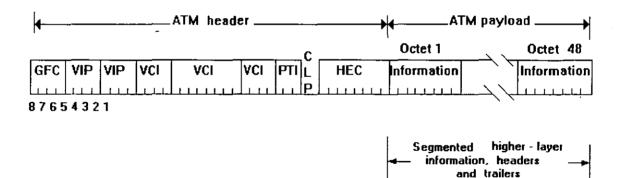
Figure 1.2 ATM cell layout
