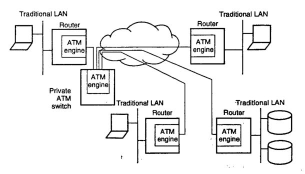
\*Figure 1.10 Private ATM technology to interconnect dispersed LAN hubs. ATM engine = the logic implementing ATM, control, and, optionally, user plane protocols.
