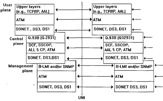
Figure 1.3 Planes constituting the ATM protocol model.
