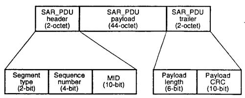
Figure 3.12 CPAAL3/4\_SAR\_PDU Sublayer format of AAL. MID = message identifier, or multiplexing identifier.
