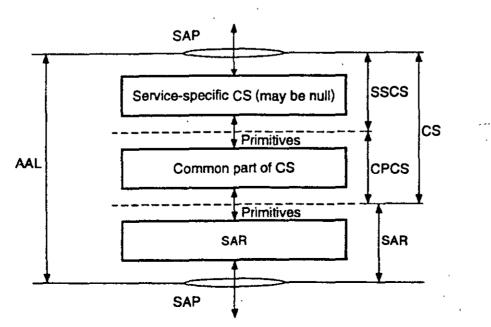
Figure 3.15 Another view of the structure of AAL Type 5.
