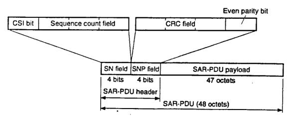
Figure 3.6 AAL Type 1 frame layout. SN = sequence number; SNP = sequence number protection; CSI = Convergence Sublayer indication.
