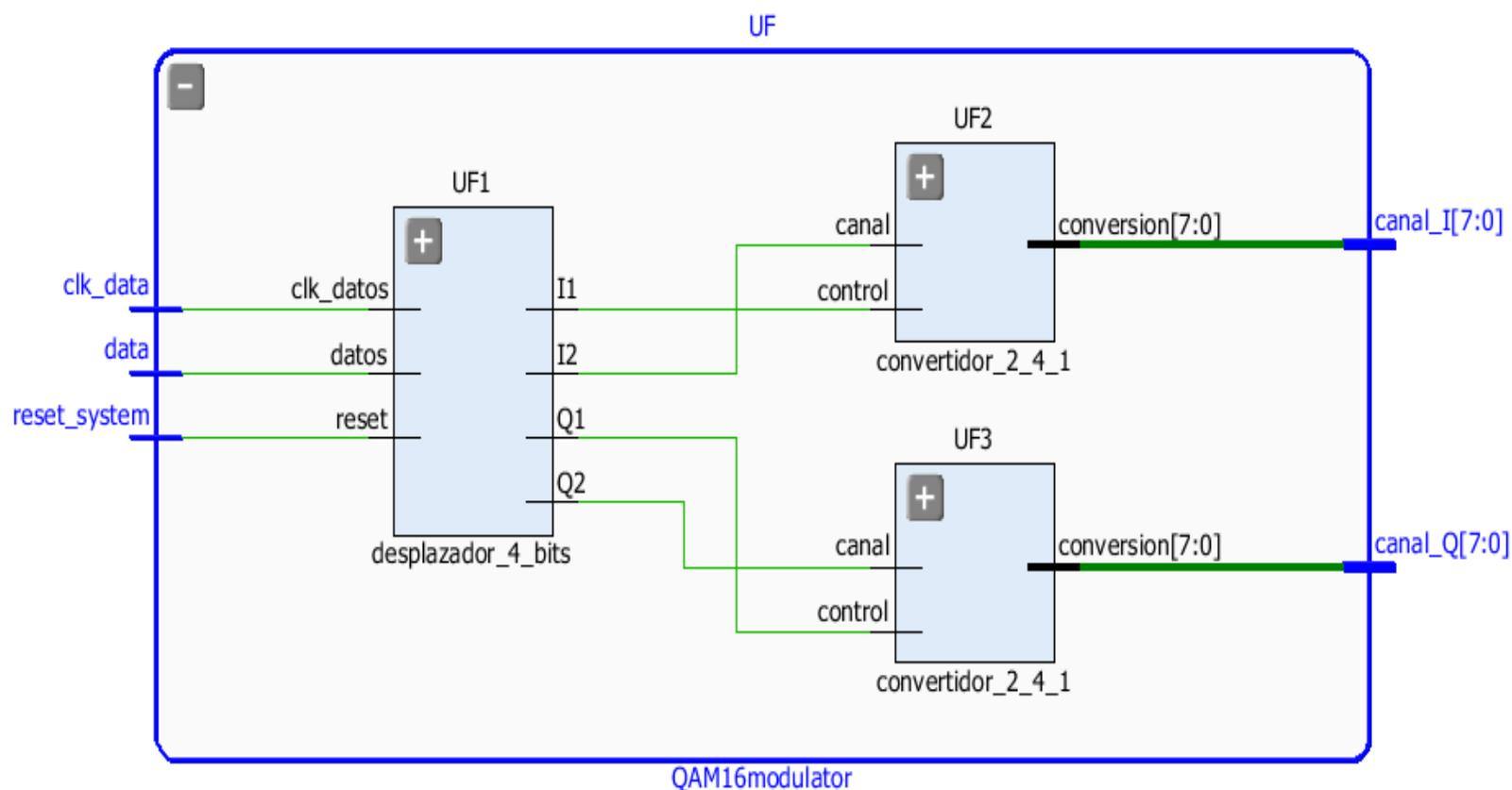
Figura 45 Top level del bloque QAM16modulator
