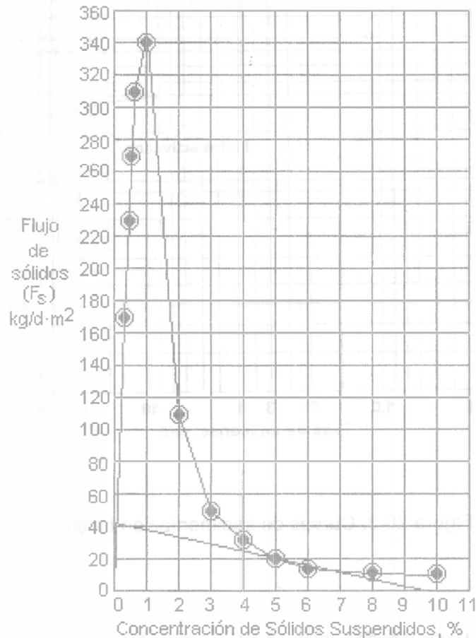
Figura 20.4. Curva flux batch.
