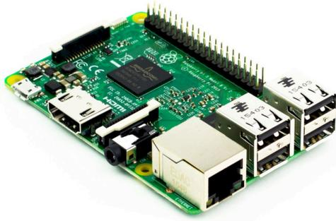
Quad Core 1.2GHz Broadcom BCM2837 64bit CPU.
