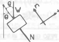
$$\sum F_t = -W \sin \theta = m \ddot{s} \quad ; \quad \sum F_n = N - W \cos \theta = m \frac{\dot{s}^2}{R} \quad \text{EN ESTE CASO } \ddot{s} = R\ddot{\theta} \quad (\text{MOVIMIENTO ANGULAR EN SENTIDO ANTIHORARIO})$$
