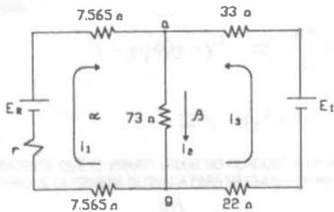
NODO a (LCK)  $i_1 - i_2 + i_3 = 0 \quad i_1 = 0.0672(\text{A})$
