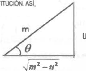
DEL TRIÁNGULO SE OBTIENEN QUE:  $u = m \operatorname{sen} \theta \Rightarrow du = m \cos \theta \, d\theta$  ;  $\sqrt{m^2 - u^2} = m \cos \theta$
