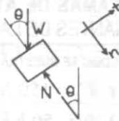
$$\sum F_t = -W \sin \theta = m \ddot{s} \quad ; \quad \sum F_n = W \cos \theta - N = m \frac{\dot{s}^2}{R} \quad ; \quad \text{dado que: } \ddot{s} = -R\ddot{\theta}$$
