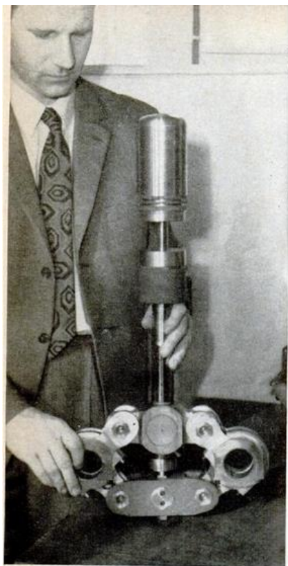
Philips engineer T. von der Ros demonstrates piston and rhombic drive action with one cylinder assembly.
