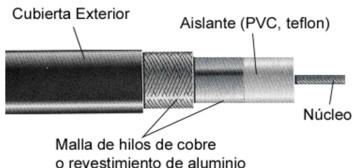
**Figura 3.33. Cable coaxial**
