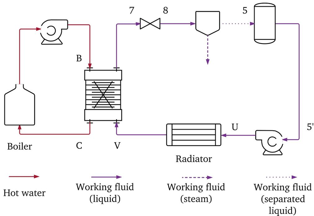
Figure 3.4: Steam generation experimental unit
