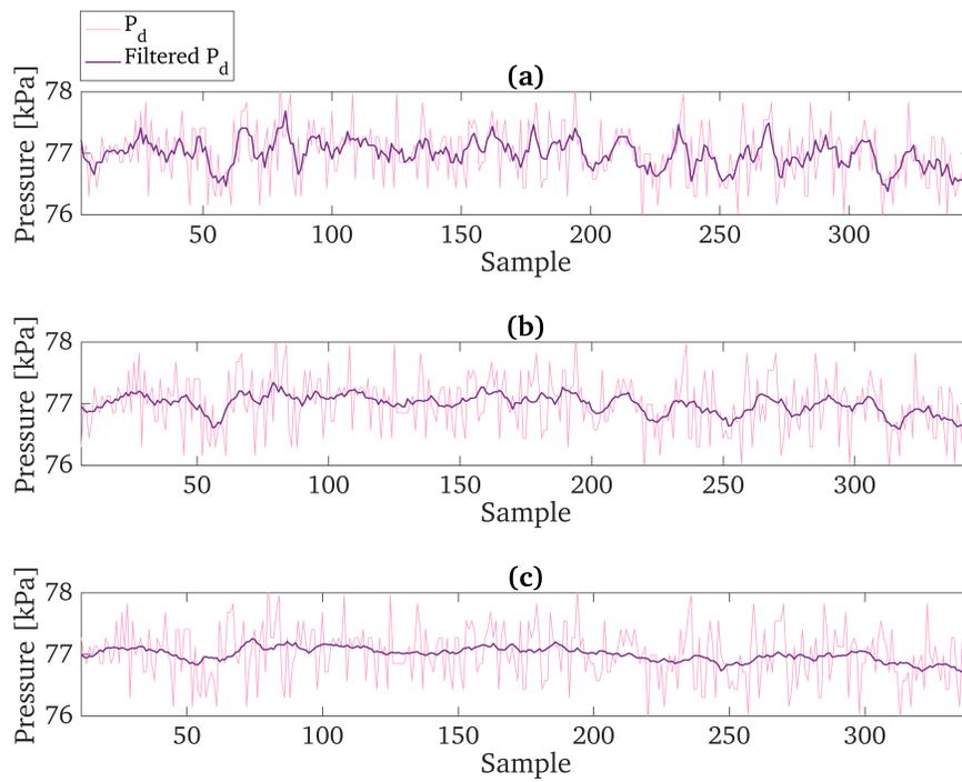
**Figure 4.28:** Filtered  $P_d$  data for different values of  $M$ . (a)  $M = 5$  (b)  $M = 11$  (c)  $M = 21$
