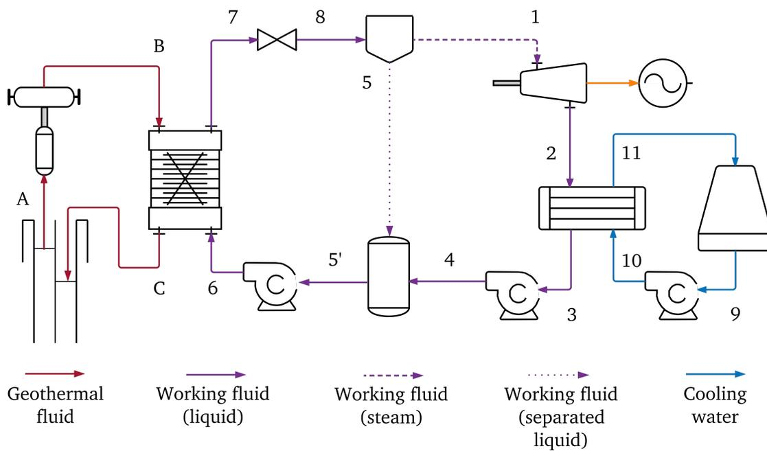
**Figure 3.2:** Thermodynamic states of Flash Evaporation Binary Cycle
