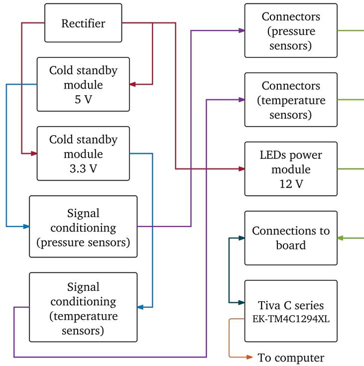
**Figure 4.3:** Hardware block diagram of instrumentation system prototype
