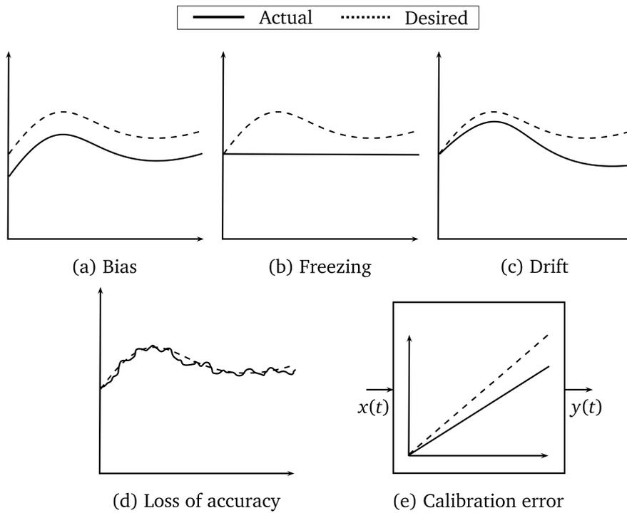
**Figure 3.7:** Fault and failures on sensors. Adapted from [116].
