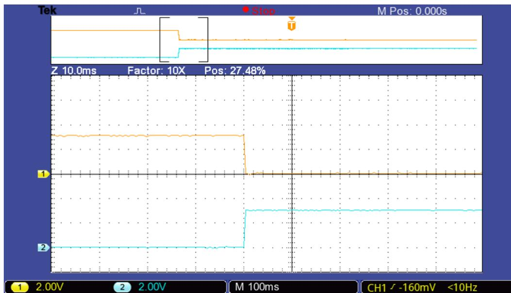
Figure 4.24: Commutation of cold standby redundant power supplies
