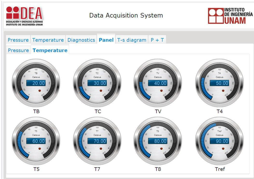
Figure 4.21: Panel for temperature readouts (simulated values)
