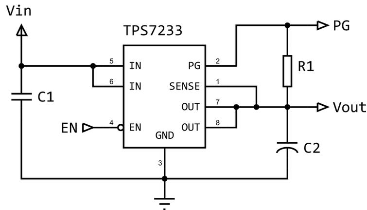
Figure 4.5: TPS7233 Low-dropout Voltage Regulator. Adapted from [130]
