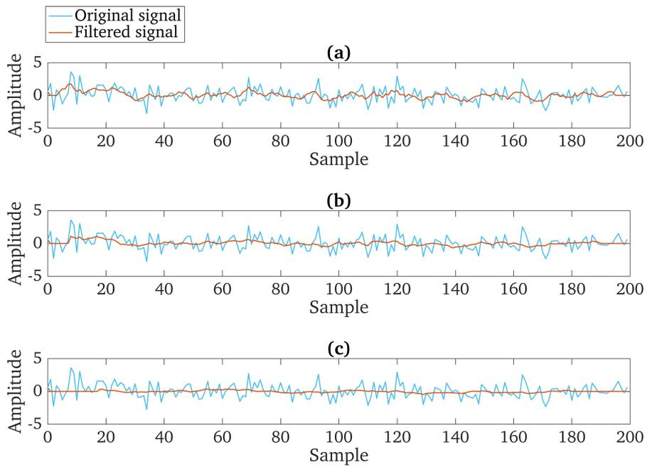
**Figure 4.10:** One-sided Moving Average Filter (a)  $M = 5$ , (b)  $M = 10$ , (c)  $M = 20$
