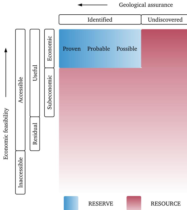
**Figure 2.3:** Categories of geothermal resources. Adapted from [22].
