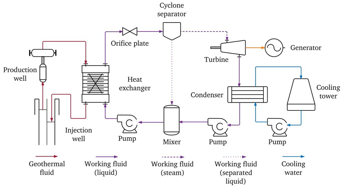
**Figure 3.1:** Flash Evaporation Binary Cycle
