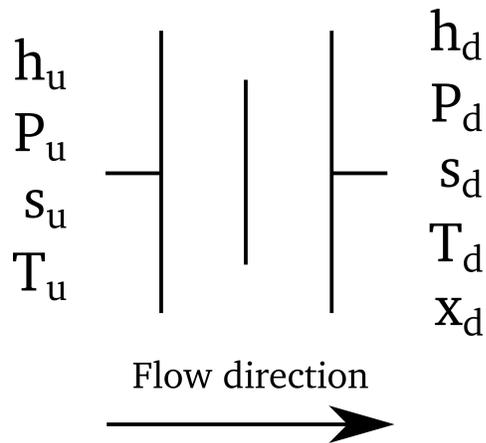
**Figure 4.13:** Thermodynamic properties of interest in orifice plate
