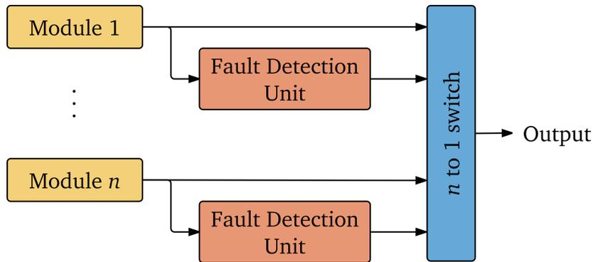
**Figure 3.8:** Cold standby hardware redundancy. Adapted from [112].
