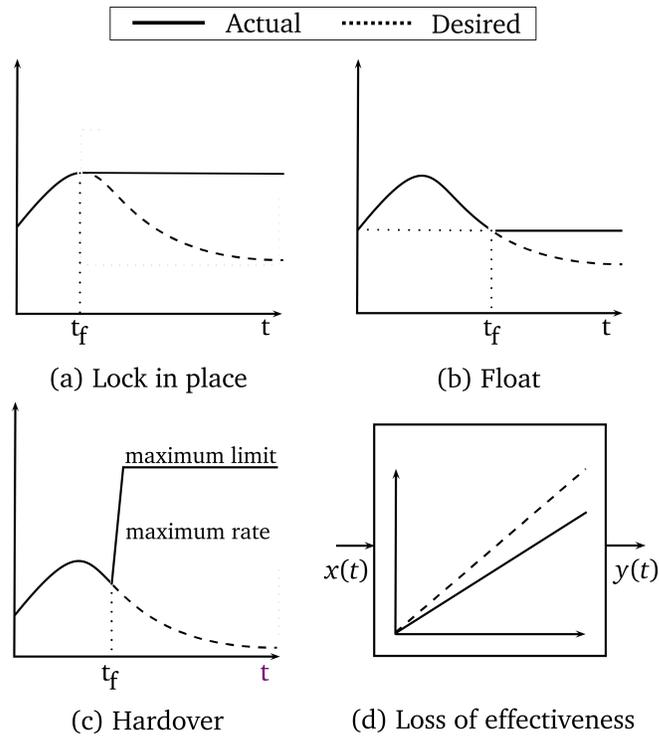
**Figure 3.6:** Fault and failures on actuators. Adapted from [116].
