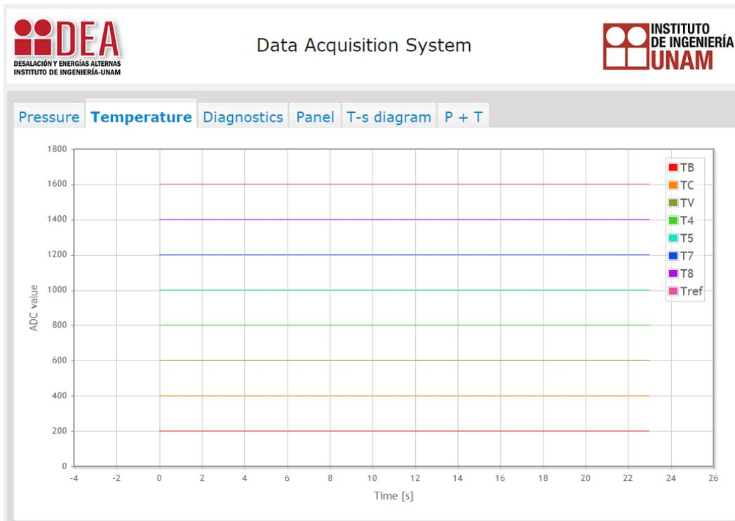
Figure 4.18: ADC values of temperature sensors (simulated values)
