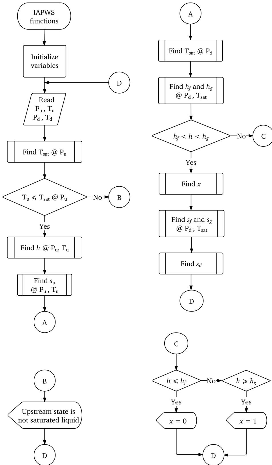
Figure 4.16: Flow chart of computation of thermodynamic properties
