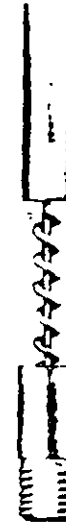
Figure . Nondamageable silver fusible element for refill units rated 10E amperes and larger. These ratings employ the silver-fusible element, strain-wire construction, which is not damaged by over loads or transient faults approaching the minimum melting current
