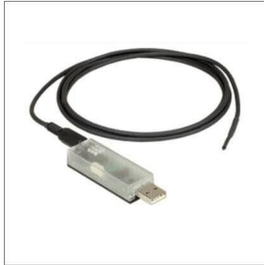
Figura 3.3: Sensor TSP01 de ThorLabs. [3]
