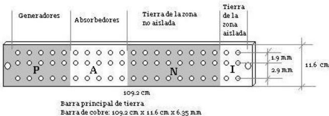
Figura 4.16 Barra principal de tierra [9] .
