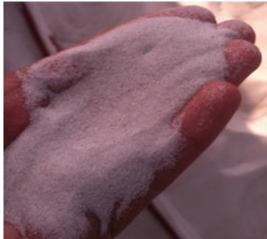
Fig. A 4.11 Tamaño de arena malla 100 (Belyadi, Fathi. Belyadi, Hydraulic Fracturing in Unconventional Reservoirs: Theories, Operations and Economic Analysis, 2017):
