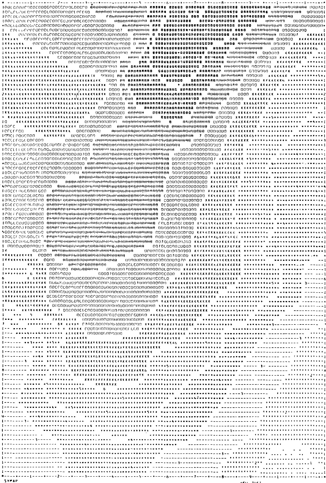
Figure 2 | Grouse Mountain, North Vancouver. Ten class intervals have been used for the contouring. The map shows the different combinations of letters used. The numbers show the location of data-points and their level. Program SYMAP, data D Mark.
