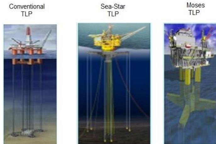
Figura 1.7 Plataforma tipo TLP (Tension Leg platform)<sup>8</sup>
