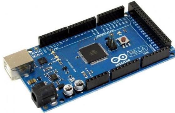
Figura 30: Arduino Mega
