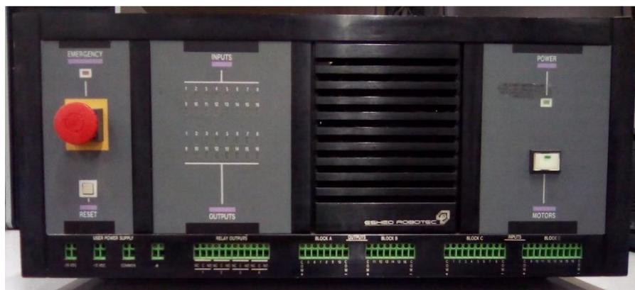
Figura 22: Controlador Eshed Robotec Controller-B ACL
