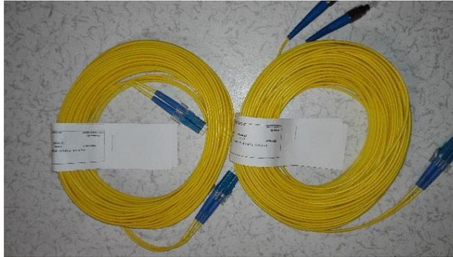
Figura 4.1. Fibras Ópticas 22 [m] FC-LC y 15 [m] LC-LC
