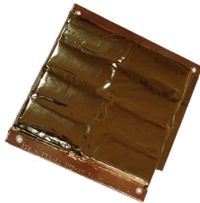
Figura 58 BA0x High Energy Density Battery Array de EXA. [64]
